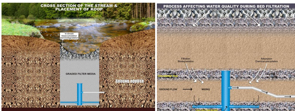
Design Drawing for low-cost, climate-resilient, and prefabricated source tapping and filtration system developed by WATSAN
