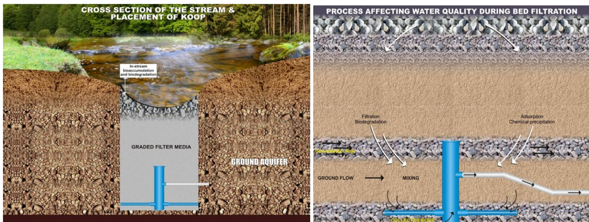
Design Drawing for low-cost, climate-resilient, and prefabricated source tapping and filtration system developed by WATSAN
