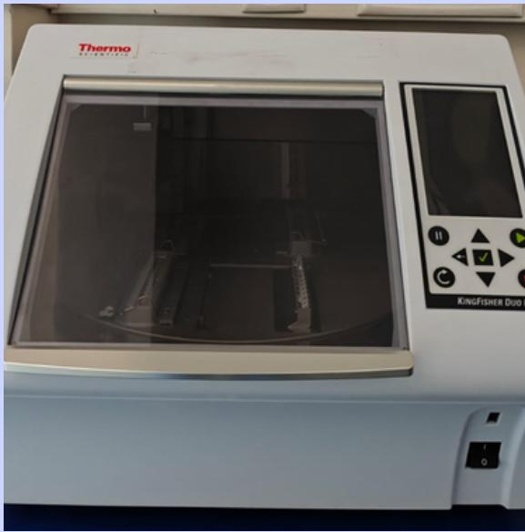
A white Thermo KINGFISHER DUO PRO automated DNA extractor. It features a large clear window on the front left showing internal components, a control panel with a small screen and buttons on the right, and a power button at the bottom right. |
