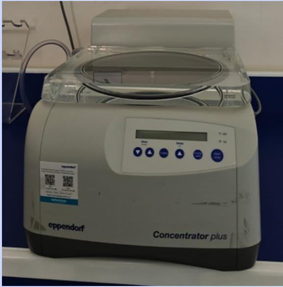
A grey Eppendorf Concentrator plus DNA concentrator. It has a clear lid, a control panel with a small screen and several buttons, and a label with a QR code and the brand name. The model name 'Concentrator plus' is visible at the bottom.   |
